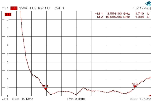
Figure 7: Measured VSWR of the proposed antenna Figure (6) and (7) show the simulated and measured VSWR of the proposed antenna respectively which is < 2 for the entire UWB range (from 3.1 GHz to 10.6 GHz).
