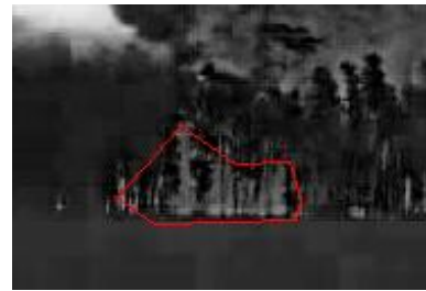
Fig. 4. Illustration of the convex hull (red line) used to evaluate the boundary roughness of the blob.
