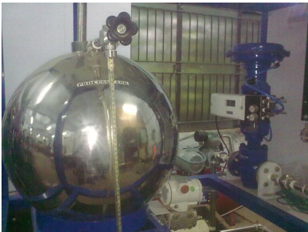
Fig 2: Real time Experimental Setup for a Spherical Tank
