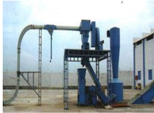
Fig 1: Pneumatic Conveying System
