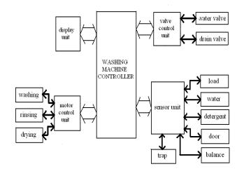
Fig. 1. Block diagram of automatic washing machine
