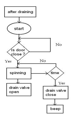
Fig. 4. Flowchart of drying module
