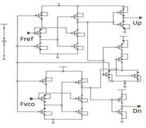
Fig. 8 Schematic diagram of Phase Frequency Detector
