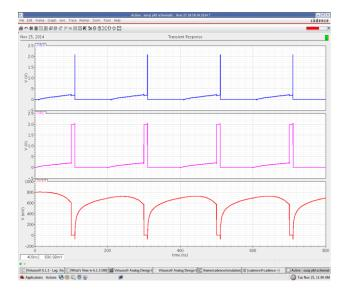
Fig.11 Transient response of PFD with Charge Pump
