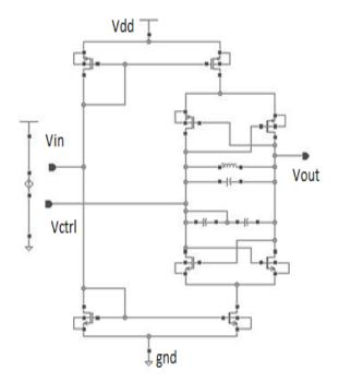
Fig. 12 Schematic diagram of VCO
