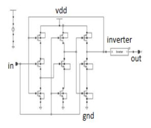
Fig.14 Schematic diagram of divide-by-2 frequency divider
