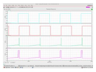
Fig. 9 Transient response of phase frequency detector
