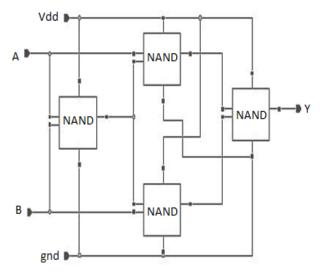
Fig.3 Schematic diagram of Phase Detector
