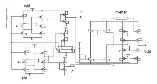
Fig.10 PFD with Charge Pump Circuit
