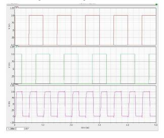
Fig. 5 Transient response at  $\Delta\Phi \approx \Pi/2$
