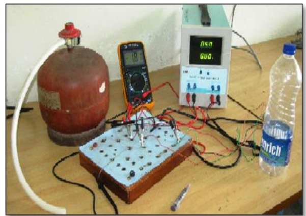
Fig 3: Experimental setup for gas sensing.
