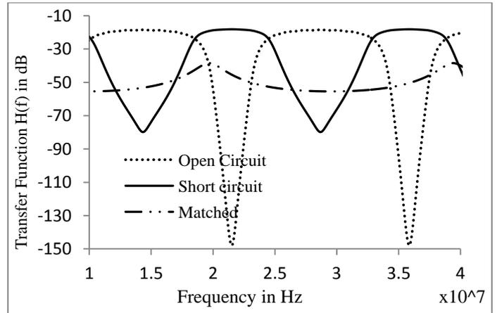
Fig7: Transfer function plot with frequency at  $Z_s=50 \Omega$ ,  $Z_L=60 \Omega$ , and  $l_{br}=5$  m, with  $Z_b=10^{10} \Omega$ ,  $0 \Omega$  and  $Z_0 \Omega$ .
