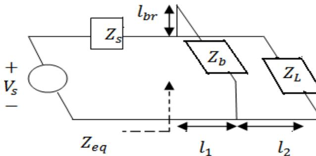
Fig 2: Transmission Line with Bridge Tap Connection.
