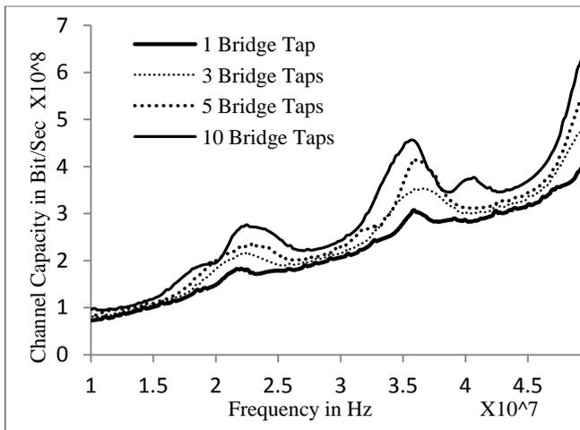
**Fig.9: Channel capacity for different number of branches at fixed direct length, load impedance, source impedance and branch load respectively.**
