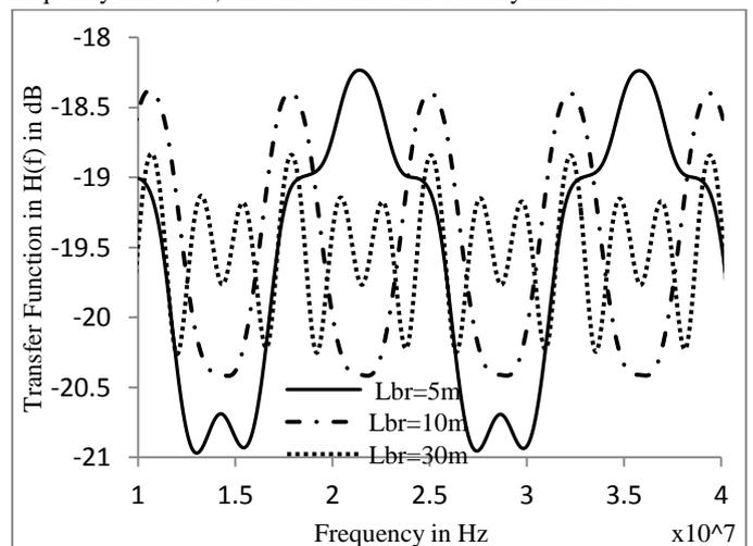
Fig 5: Transfer function plot with frequency at  $Z_s=30 \Omega$ ,  $Z_L=30 \Omega$ ,  $l_1=20\text{m}$ ; and  $l_2=20\text{m}$ .
