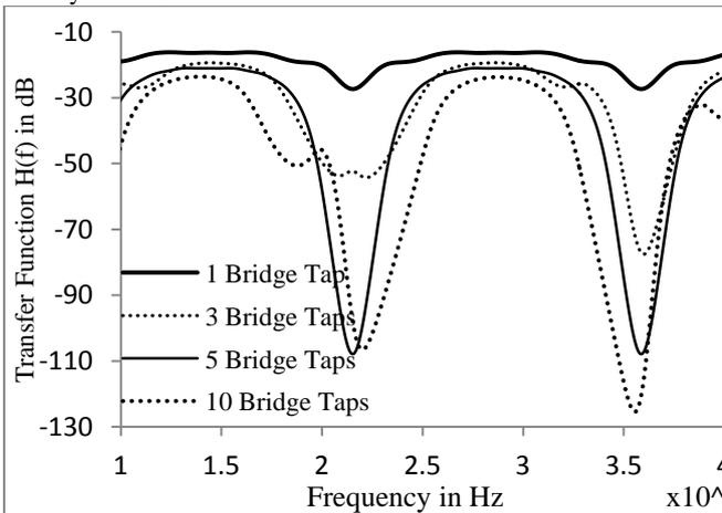
Fig 6: Transfer function plot with frequency at  $Z_s=50 \Omega$ ,  $Z_L=60 \Omega$ , and  $l_{br}=5$  m, with  $Z_b=500 \Omega$ .
