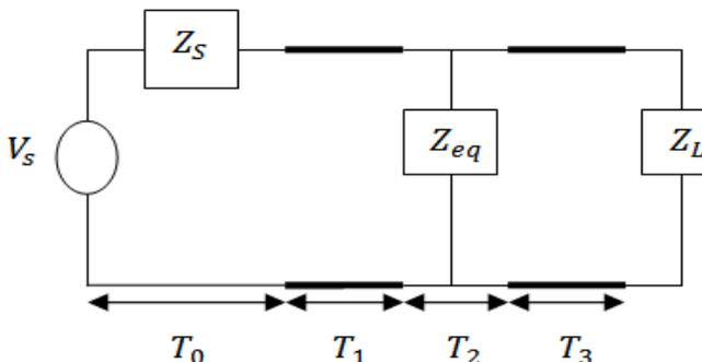
Fig 3: Equivalent Network Circuit for Bridge Tap Connection.
