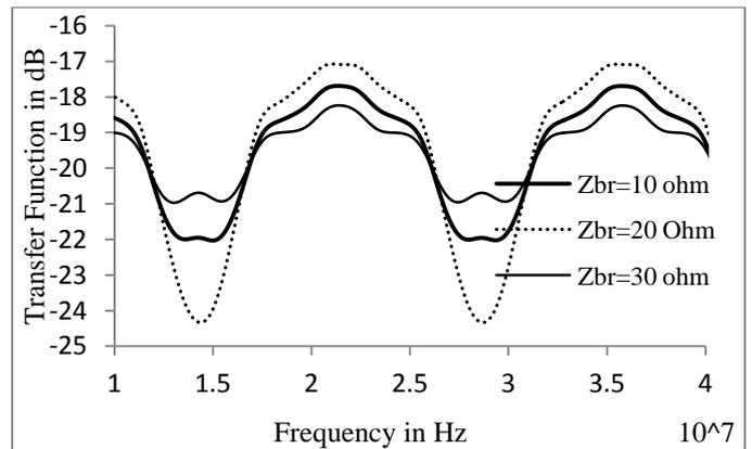
Fig 4: Transfer function plot with frequency at  $Z_s=30 \Omega$ ,  $Z_L=30 \Omega$ ,  $l_1=20\text{m}$ ;  $l_2=20\text{m}$ ; and  $L_{br1}=5\text{m}$ .
