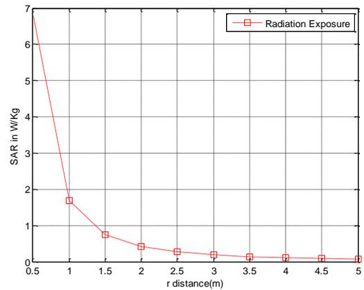
**Fig 5: SAR vs. distance in human head model at frequency 925MHz**
