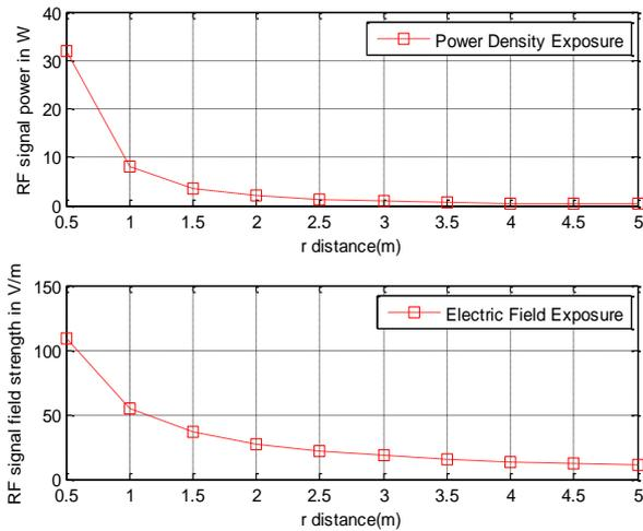
**Fig 3: Power density and Electric field over distance for GSM 925 MHz application compared to the limit for public exposures**
