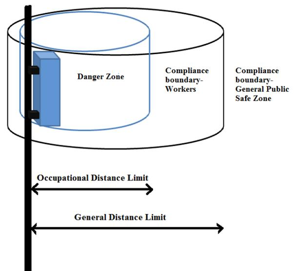
Fig 2: Proposed system model for safe limit identification
