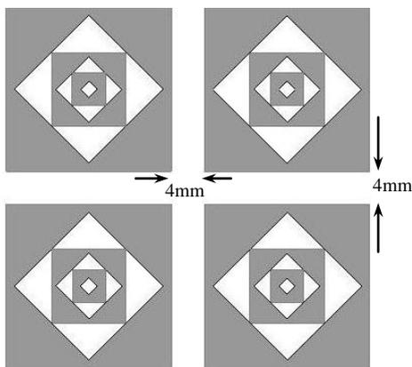
Fig 4: FSS showing four patch element and Spacing between adjacent patches.
