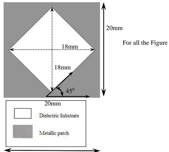
Fig 1: Basic design of the FSS Patch
