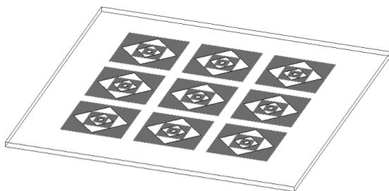
Fig 5: FSS showing two dimensional array of patch on dielectric substrate.
