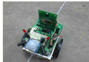
Fig. 10 (a) Boe-bot sending current co-ordinate through Bluetooth
