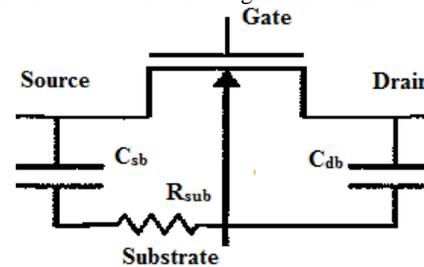
Fig. 1 Reverse biased junction Capacitance of MOSFET
