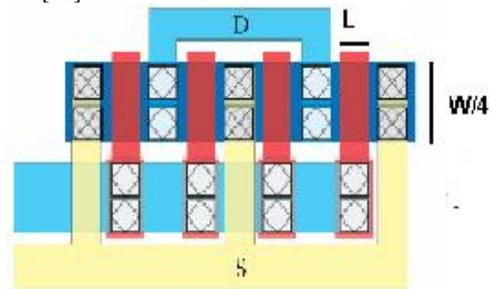
**Fig.5 Multifinger gate structure**
