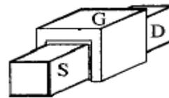
**Fig. 6 Typical triple gate structure**
