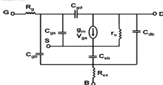
Fig.3 The small signal equivalent circuit of CMOS device
