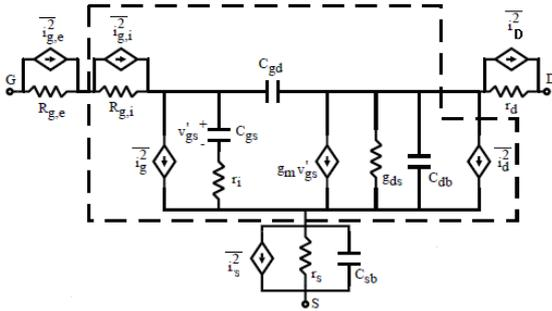
**Fig.4 A complete small signal representation of RF CMOS device** [2]
