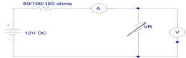
Figure 13: Circuit diagram of apparatus used for verification of maximum power transfer theorem
