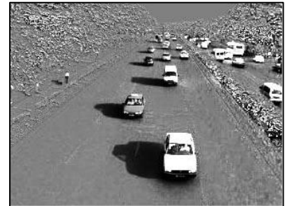
(f) Converting the resultant video frame to grayscale image
