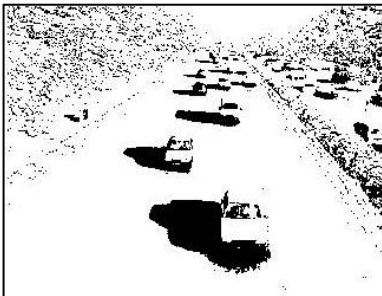
(g) The white pixels indicate the pixels with value greater than the threshold
