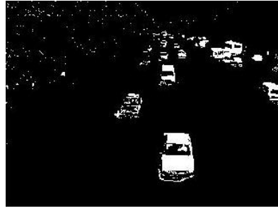
(h) The resultant frame after thresholding
