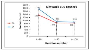
Fig 8: Network of 100 mesh routers cost
