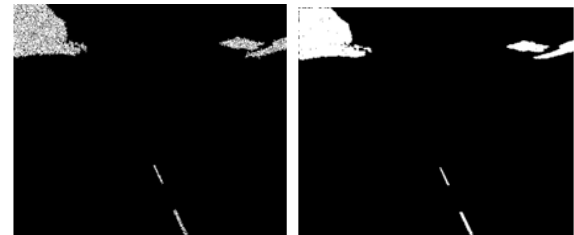
Fig.2.4 (a): without filter Fig.2.4(b): with median filter
