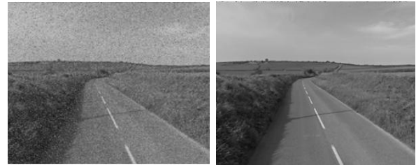
Fig.2.2(c): with wiener filter Fig.2.2(d): with HMF
