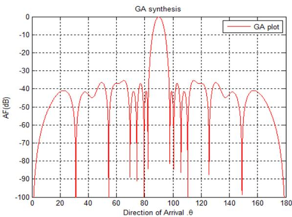
**Fig 6a: Optimized Radiation pattern with reduced sidelobe level for N=24 elements array for GA method.**
