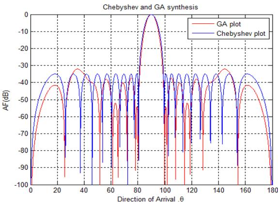
**Fig 5b: Optimized Radiation pattern with reduced sidelobe level for N=20 elements array for GA & Dolph Chebyshev methods**
