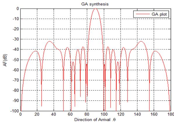
**Fig 5a: Optimized Radiation pattern with reduced sidelobe level for N=20 elements array for GA method.**
