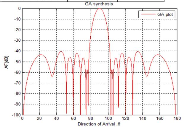
**Fig 4a: Optimized Radiation pattern with reduced sidelobe level for N=16 elements array for GA method**
