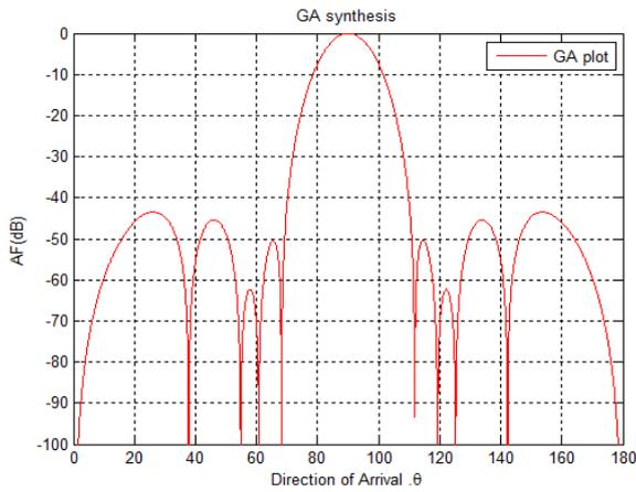
**Fig 3a: Optimized Radiation pattern with reduced sidelobe level for N=10 elements array for GA method.**
