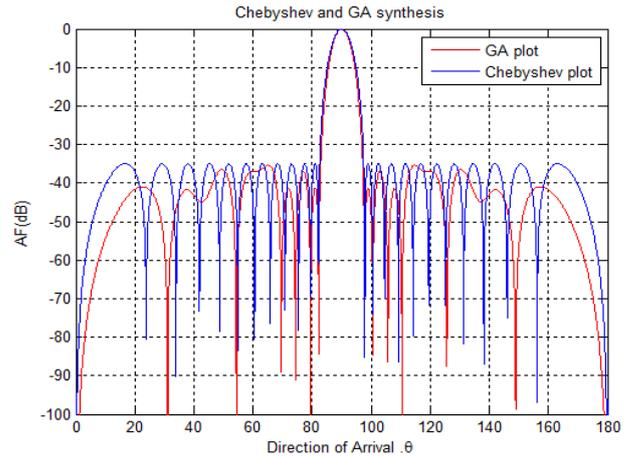
**Fig 6b: Optimized Radiation pattern with reduced sidelobe level for N=24 elements array for GA & Dolph Chebyshev methods**
