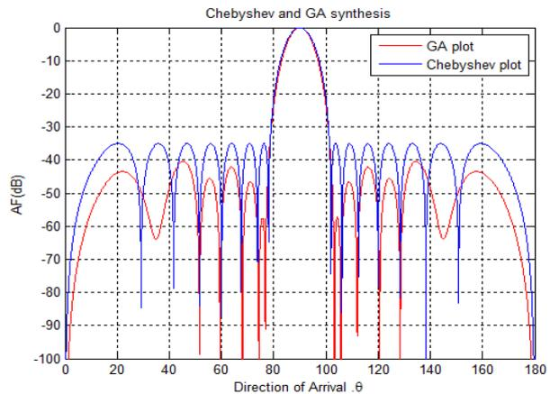
**Fig 4b: Optimized Radiation pattern with reduced sidelobe level for N=16 elements array for GA & Dolph Chebyshev methods**
