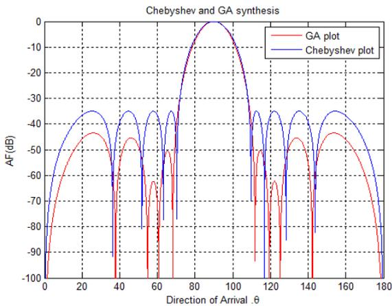
**Fig 3b: Optimized Radiation pattern with reduced sidelobe level for N=10 elements array for GA & Dolph Chebyshev methods**
