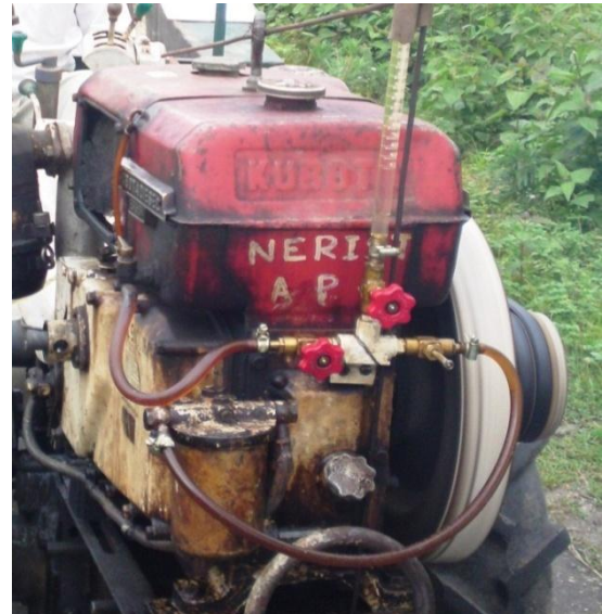
Fig 7: Fuel measuring setup mounted on power tiller
