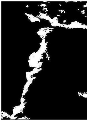
Fig. 4. Local threshold segmented image
