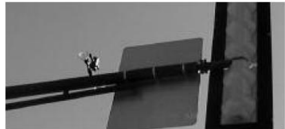
Fig 2: Infrared-based preemption systems, the infrared receiver should be mounted on a high place at the traffic light. The infrared transmitter and receiver should be within an effective line of sight from each other in order to operate properly [1].
