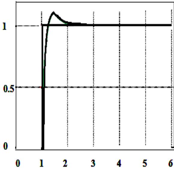
**Figure 8**The response of the system for LQR.
