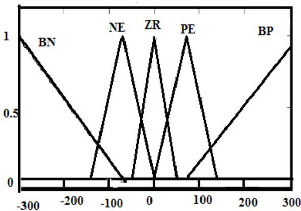
**Figure 5 Rate of error membership functions.**
