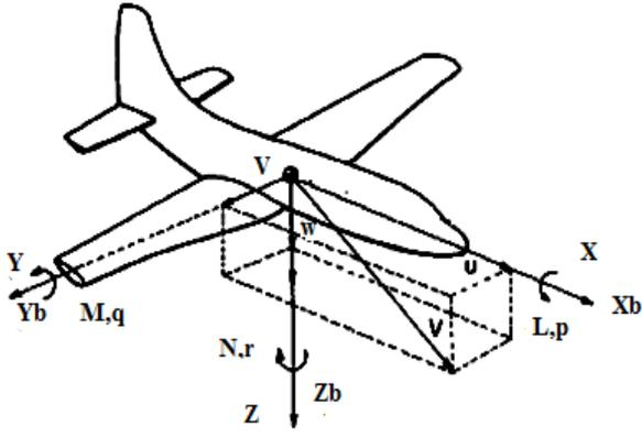
**Figure 2. Definition of forces, moments and velocity components in a body fixed frame [1].**
