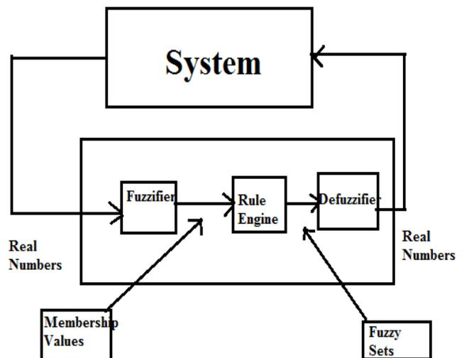
**Figure 3. The basic structure of fuzzy logic based controlle**
