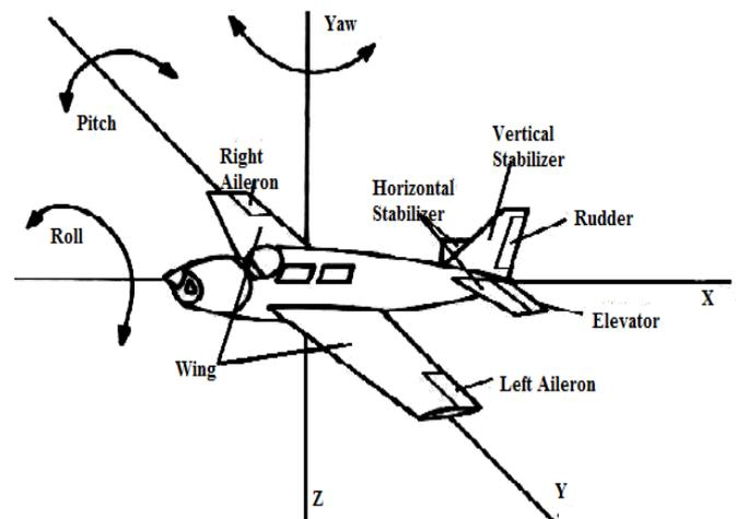
Figure 1. Yaw, Roll & Pitch motion of Aircraft [10].
