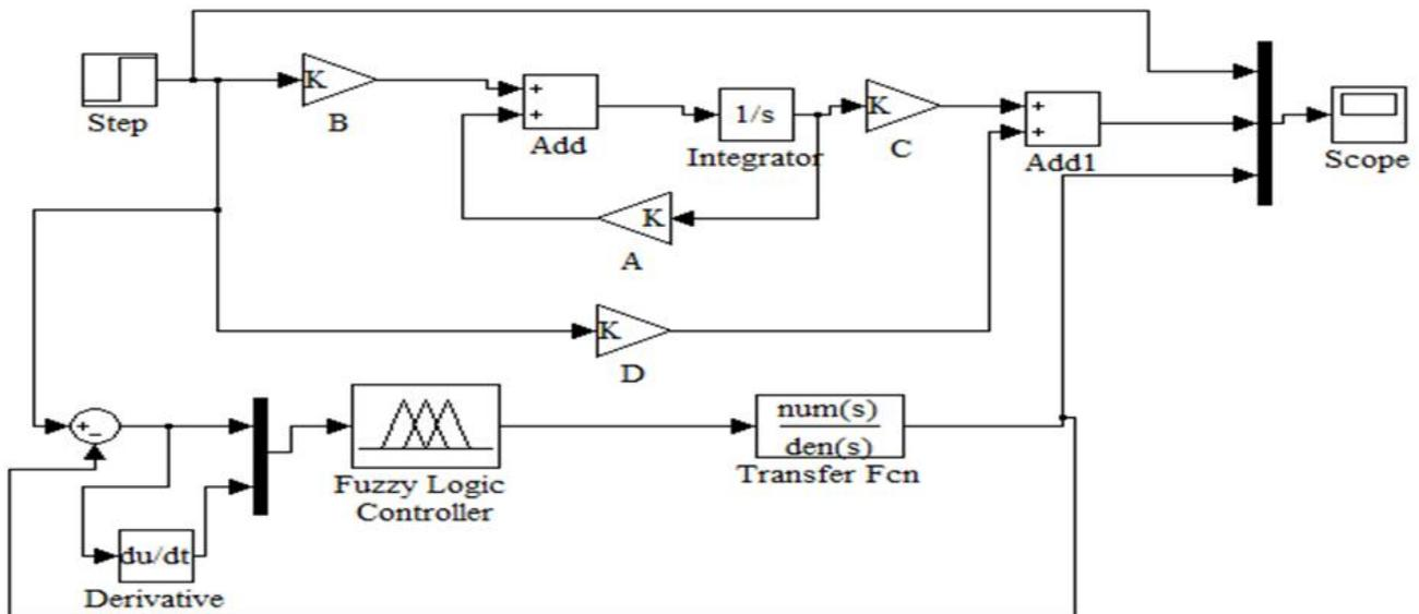
**Fig 10 Matlab/Simulink model for the roll control system**
