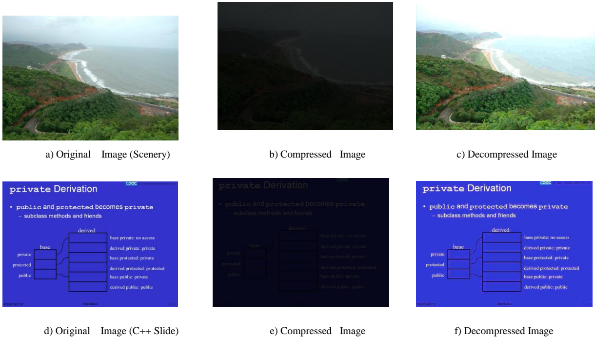
Fig 2: Compression and Decompression of images using JPEG format 1440x900 Resolution
