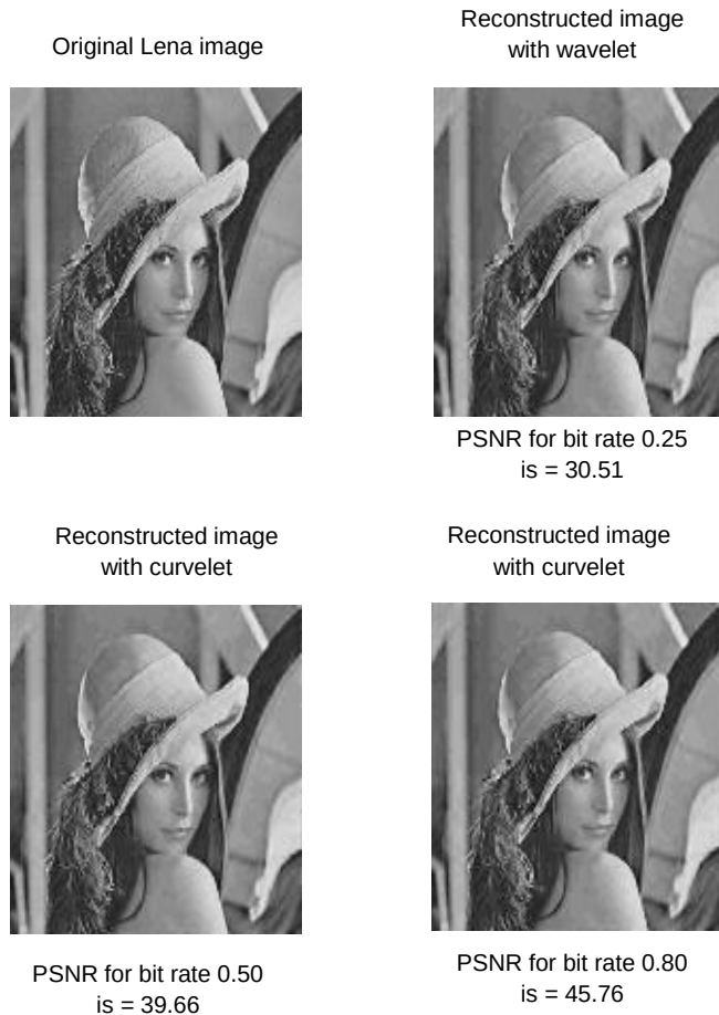
Fig 5: Fractal -Wavelet & fractal -Curvelet Transformed Lena image for various bit rate
