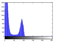
Figure 15. y) Histogram plot after the removal of non-uniform background indicating uniform variation in the image corresponding the equal distributions of probability at the output.
