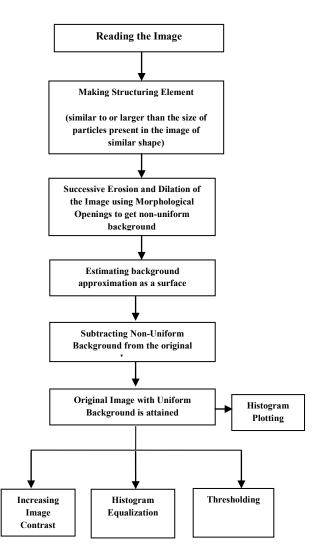
Fig.11: Algorithm Designed for non-uniform background removal for particle analysis and image enhancement
