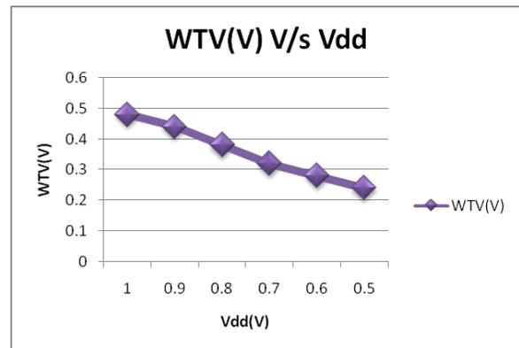
Fig. 5 Write Stability: WTV with varying V<sub>dd</sub>.
