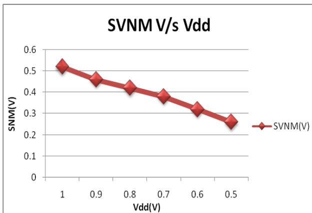
Fig. 3 Read Stability: SVN<sub>M</sub> V/s V<sub>dd</sub>
