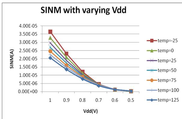
Fig. 4 Read stability: SIN<sub>M</sub> V/s V<sub>dd</sub>
