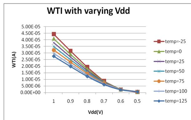
Fig. 6 Write Stability: WTI with varying V<sub>dd</sub>
