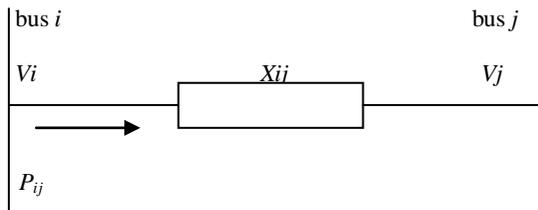
Figure 1. Power ( $P_{ij}$ ) flow between buses *i* and *j*
