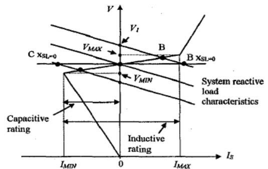
Figure 2 . Voltage- Current Characteristics of SVC
