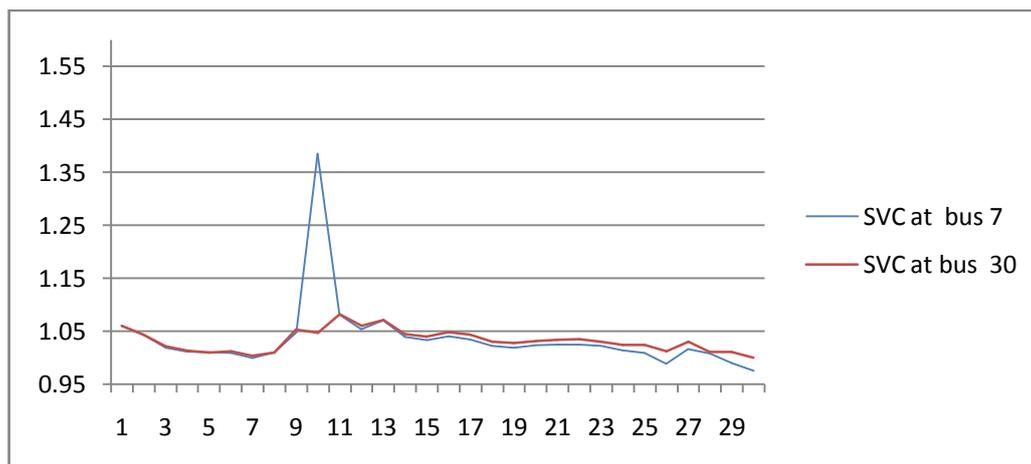
**Figure 4. Voltage deviation when randomly the load is varied**
