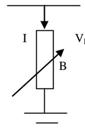
Figure 3. Variable Shunt Susceptance Model
