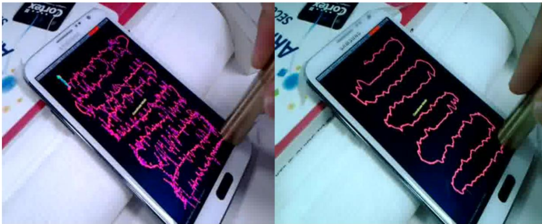
Figure 9: Qualitative performances of proposed algorithms on Galaxy S4 Handset for finger drag in the presence of high amount of charger noise. Left side of the figure depicts output of Modified Moving Average Filter where as right side of the figure depicts output of Proposed Three Stage Filter
