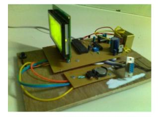
Fig 10. Side view of the developed system board.
