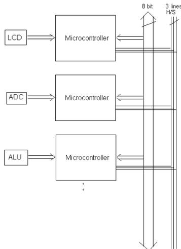
Microcontrollers are versatile integrated circuits typically incorporating a microprocessor, memory, and I/O ports on a single chip. These self-contained units are central to embedded systems design where low-cost, dedicated processors are often preferred over general-purpose processors. Some embedded designs may incorporate several microcontrollers, each with a specific task. Efficient communication is central to such systems.
