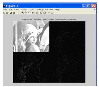
Figure 1. One level Haar wavelet Decomposition
