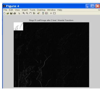
Figure 2. Three level Haar wavelet Decomposition of Lena image.
