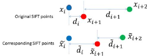
Figure 3: Vertical seam estimation using  $x$ -coordinates of matched SIFT point pairs
