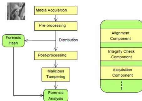
Figure 2: Flowchart of media processing and modular design of forensic hash
