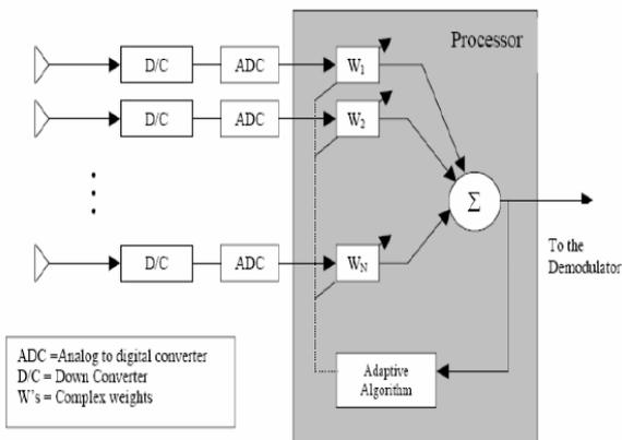
Figure 1: Functional block diagram of an adaptive array system. [1]
