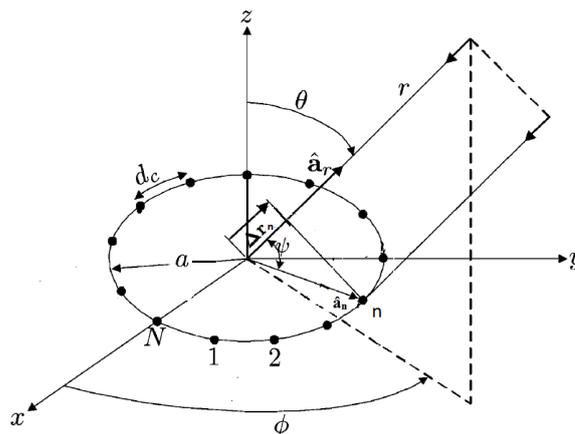
Figure 3: Geometry of an N-element circular array.[6]
