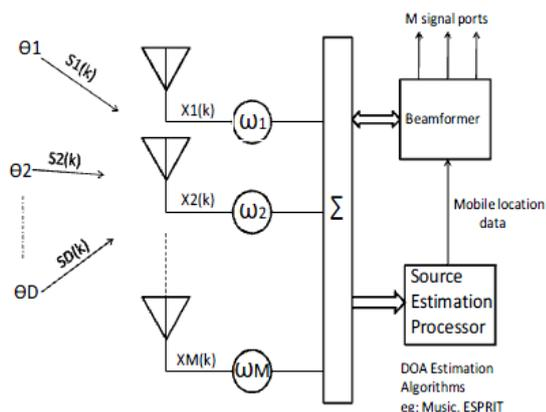
Figure 4: M element antenna array with D arriving signals.[10]
