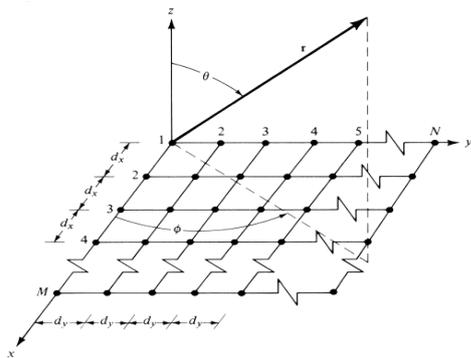
Figure 2 Planar array geometry.[4]
