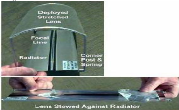
Fig.6 Single Cell Stretched Lens Array enables low mass high efficiency power generation
