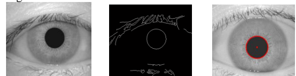
Figure 1 Steps involved in detection of inner pupil boundary
