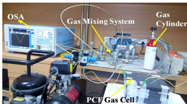
Fig.3. Gas sensing Lab Experimental set up
