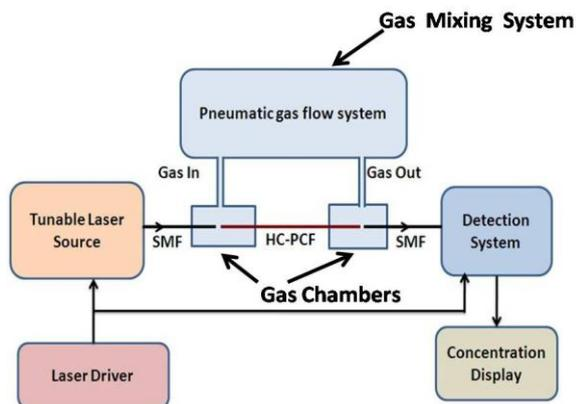
Fig.2 Schematic diagram of HC-PCF gas sensor
