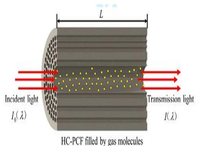
Fig.1. Schematic diagram of absorption principle of HC-PCF gas sensor
