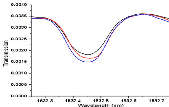
Fig.4 Transmission Profile of Different Concentration of Acetylene gas through HC-PCF gas cell
