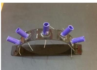
Fig 3: Light Dependent Resistors in Cylindrical Covering
