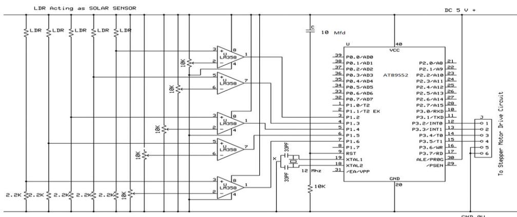
Fig 2: Schematic of Solar Tracker Circuitry
