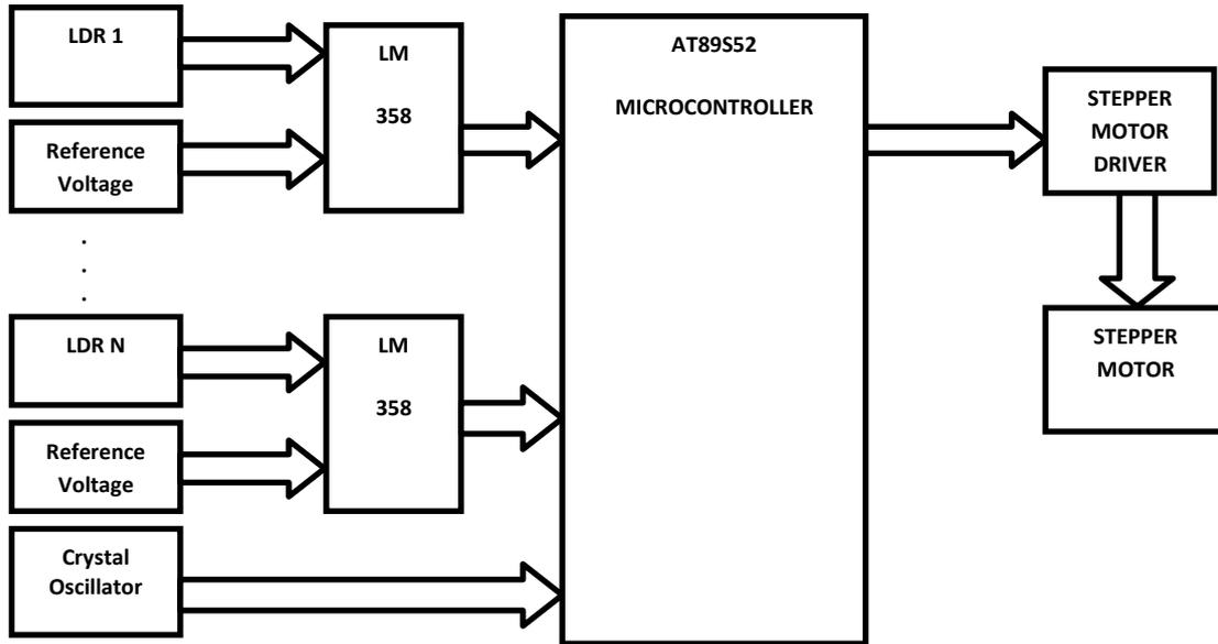
**Fig 1: Block Diagram of the Solar Tracker**
