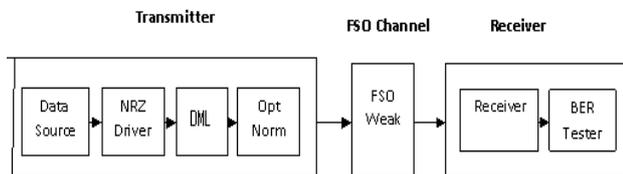
Figure 1. Block diagram of FSO.
