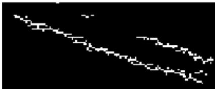
**Figure 12: Horizontal Sobel edge detection with discontinuous edge pixels.**
