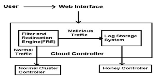
Fig 4: Cloud Controller with FRE and Log Storage System
