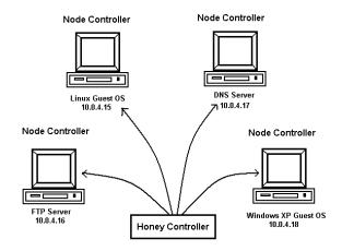
Fig 3: Honey Controller with Virtual Instances
