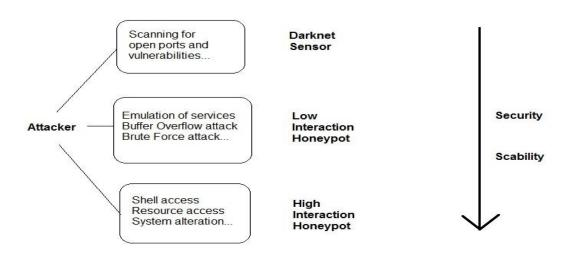
Fig 1: Different Honeypot architectures to collect different phases of network attacks
