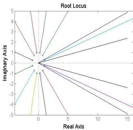
Fig 4: Root locus for fractional order model
