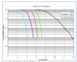
Figure.7 CCDF of PAPR reduction performances with different N values while M is fixed with PTS
