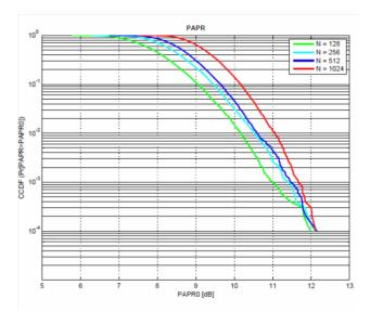
Figure.6 CCDF of PAPR reduction performances with different N values while M is fixed without PTS.
