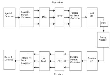
Figure. 2 Block diagram of OFDM System
