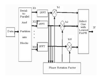
Figure.5 Block Diagram of Partial Transmit Sequence
