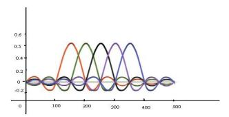
Figure.1 OFDM Spectrum
