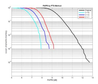
Figure.8 CCDF of PAPR reduction performances with different V values while N is fixed at 128
