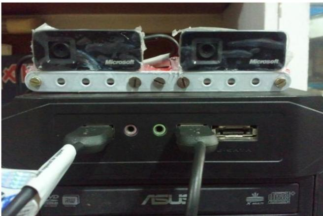
Fig 11: Front view of the stereo Rig
