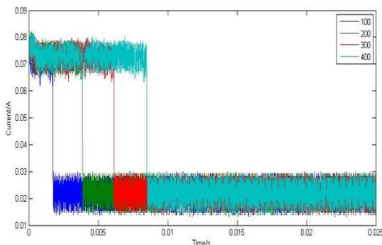
**Figure 6: Current Measurements for Merge Sort in Xilinx Platform for Different Iterations**
