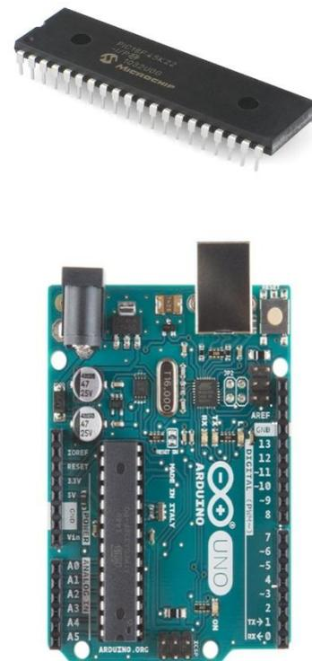
Fig. 1: Microcontroller Vs Arduino Uno
