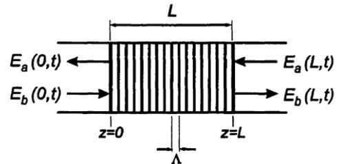
Fig. 2. Propagating waves in Bragg grating
