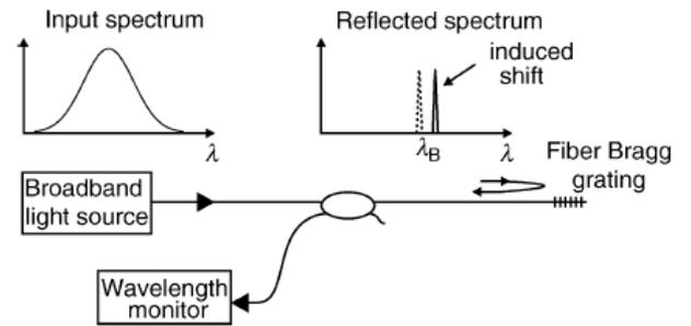
Fig 1. Basic reflective FBG sensor system
