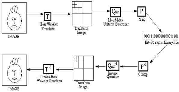
**Figure 2: Haar Wavelet Transform Architecture**
