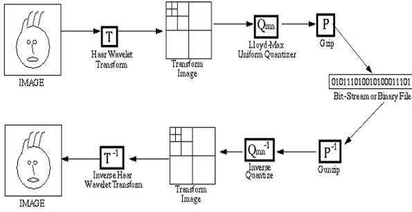
**Figure 2: Haar Wavelet Transform Architecture**
