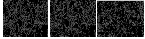
Fig 2: Canny edge detection of red and blue channels by taking green channel as reference and of green channel by taking red channel as reference
