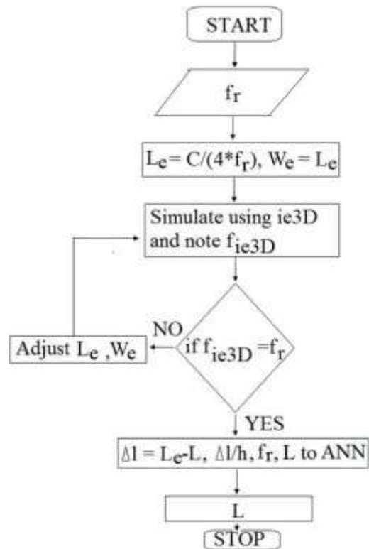
Fig 2 Flowchart for calculating shorted RMSA length
