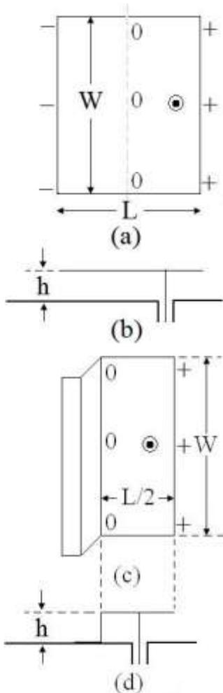
Fig 1: (a) Top and (b) views of RMSA and (c) top and (d) side views of shorted RMSA
