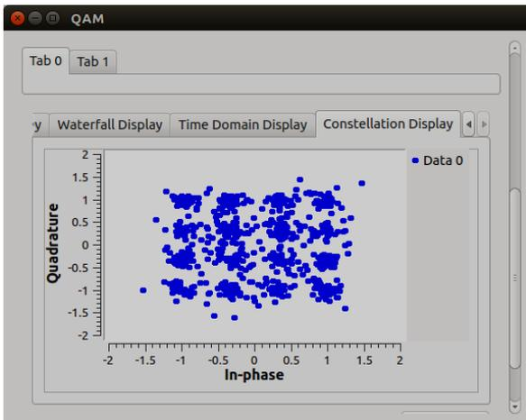
**Fig 7: Constellation plot of QAM**
