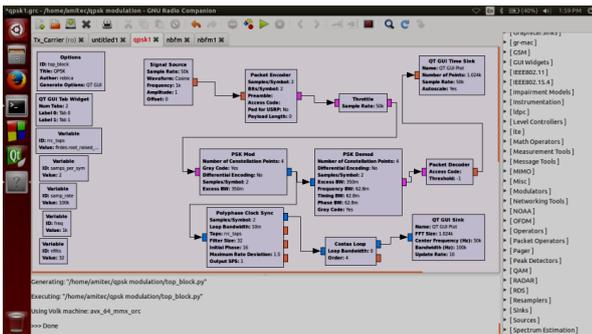
Fig 1: GRC block diagram of QPSK
