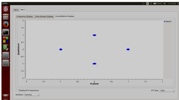
Fig 3: Constellation plot of QPSK
