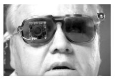
Figure2. Blind volunteer with sub-miniature TV camera mounted on the right lens of his sunglasses, and the laser-pointer (position monitor) on the left temple piece.
