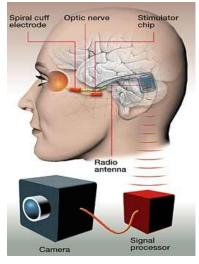
Figure6. The Optic Nerve Implant [5]
