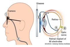
Figure4. The Bionic Eye Implant [5]
