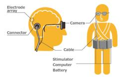
Figure 5. The Cortical Implant [5]
